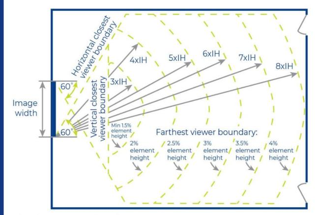
Viewing Parameters for BDM No scale. IH = Image Height. Image Height based on 16:9 (1.78:1) aspect ratio.
