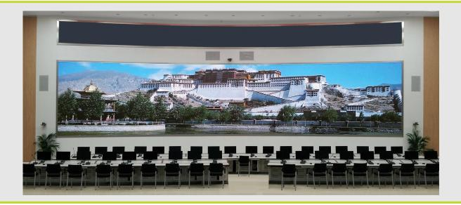
The VDL Supernova Infinity is a modular screen system featuring Supernova's advanced ambient light-rejecting TrueALR optical screen technology for exceptional image quality at a fraction of the purchase costs, running costs and environmental impact of dvLED.
